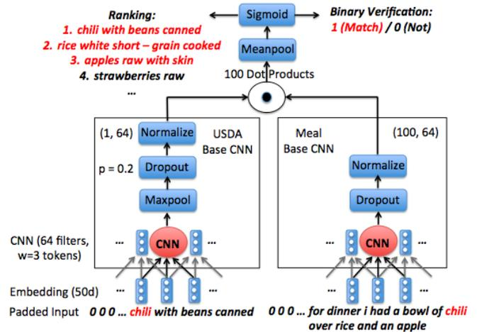
Fig. 2. Architecture of our CNN model for predicting whether a USDA food entry is mentioned in a meal description.
