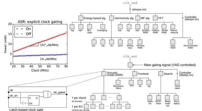
Fig. 14. Clock gating hierarchy: VAD clock domain (top) and ASR clock domain (bottom). The impacts of explicit clock gating are shown at left.
