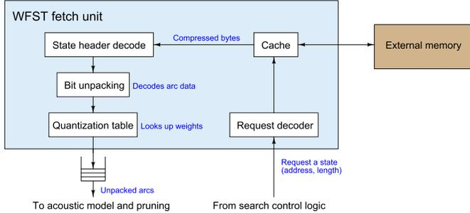
Fig. 8. WFST fetch architecture with caching and model compression.
