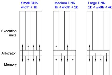
Fig. 4. EUs and local memory are grouped into chunks that can be reconfigured for different network sizes.
