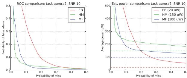
Fig. 12. Left: ROC of each VAD on Aurora2 task at 10-dB average SNR. Right: estimated system power derived from ROC at 5% speech duty cycle. This plot uses early (conservative) estimates of VAD power for each algorithm, as shown in the inset and dashed lines, and 1-mW downstream system power.
