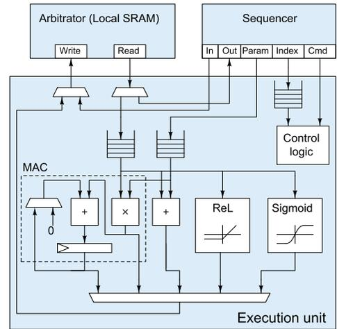
Fig. 5. EU block diagram (pipelining, addresses, and control signals not shown).
