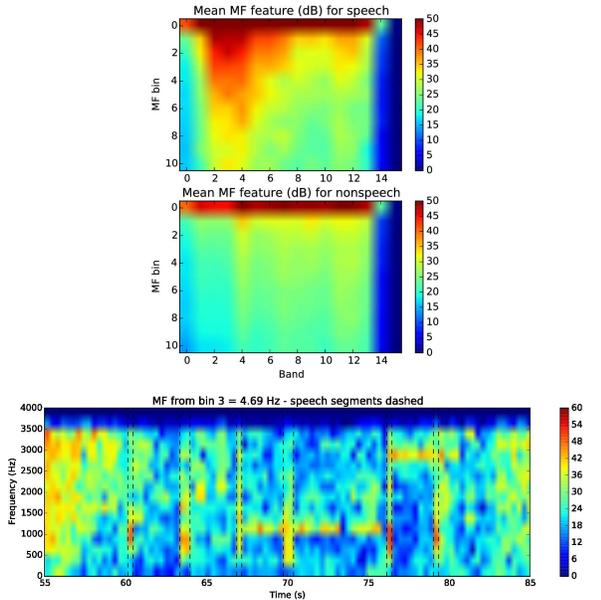
Fig. 11. Examples demonstrating the separability of MF features in noisy conditions: mean MF matrix for speech and non-speech (top), and 4-Hz MF spectra (bottom), at 0-dB SNR. Dashed vertical lines: speech segments.
