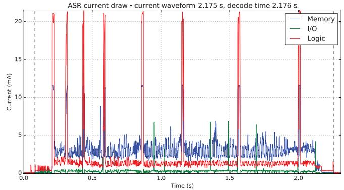
Fig. 17. Current measurement of each power supply during ASR decoding of an utterance from the food diary data set. Variations in search workload are visible as different lengths of decoding time between acoustic model evaluations (periodic spikes), which occur after every 32 frames (320 ms) of input.
