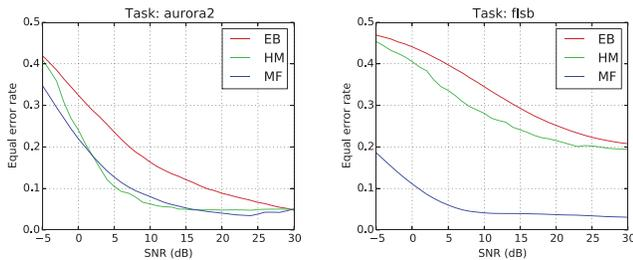
Fig. 13. EER versus average SNR on Aurora2 task (left) and Forklift/Switchboard task (right).
