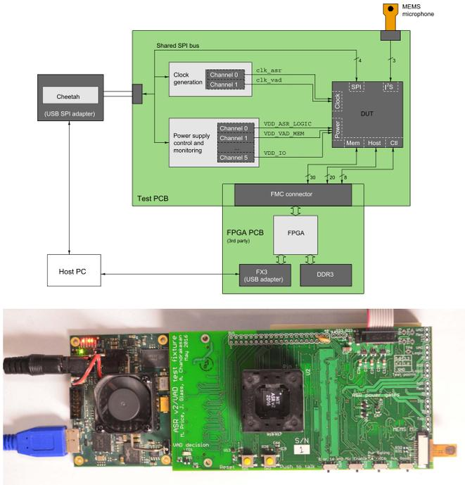
Fig. 16. Block diagram (top) and photograph (bottom) of test PCB stack integrating power supplies and functional test interfaces.
