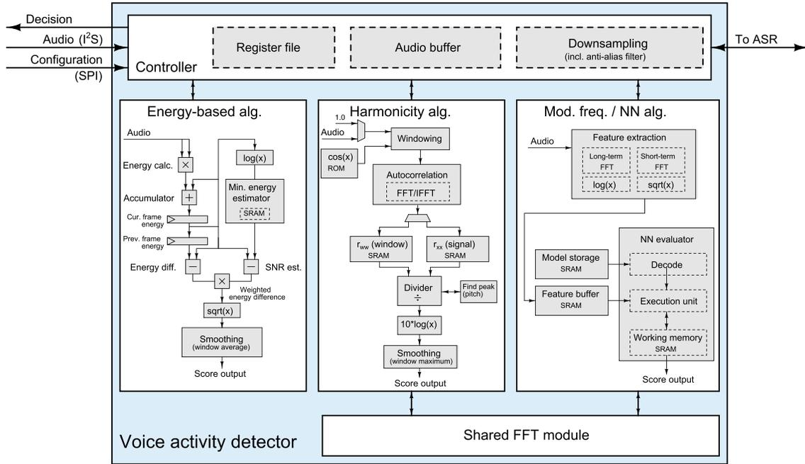
Fig. 9. Block diagram of VAD that can selectively enable EB, HM, and MF algorithms. Score computation pipelines for each module are shown.
