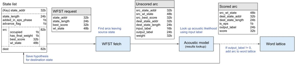
Fig. 7. Data fields for state list entries and in-flight hypotheses. The architecture is designed to preserve memory locality.
