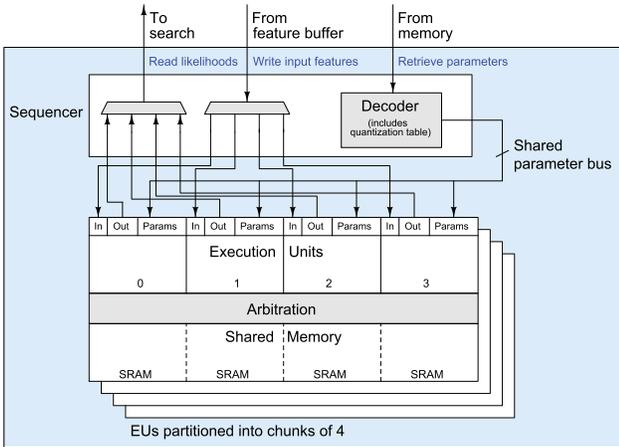
Fig. 3. Block diagram of SIMD NN evaluator, relying on a shared sequencer and 32 EUs. External memory access is read-only due to internal storage of activations.
