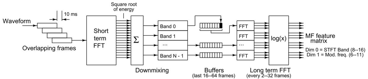
Fig. 10. MF feature extraction: the short-term FFT bins signal energy by band, and the long-term FFT bins signal energy by MF.
