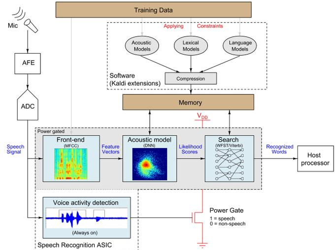
Fig. 1. Conceptual illustration of speech recognizer with voice-activated power gating. Training is performed off-line to prepare models stored in an external memory and used by search and acoustic modeling within the chip. This paper describes the digital ASIC and supporting software components surrounded by dashed boxes.
