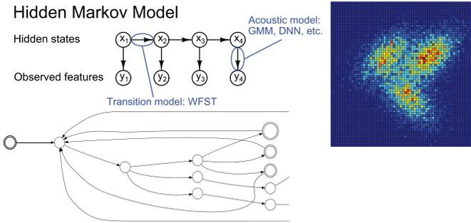
Fig. 2. HMM formulation of ASR. Searching for word hypotheses requires two types of statistical models: a WFST for transitions between hidden states, and an acoustic model for the observations (feature vectors) conditioned on each hidden state.
