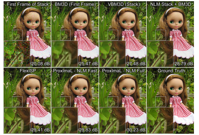
Figure 9: Comparison of image priors for burst denoising & demosaicking. For this simulation, a non-local means (NLM) prior outperforms the BM3D prior. The approximate NLM implemented in OpenCV is faster than, but not quite as good as, a full implementation.
