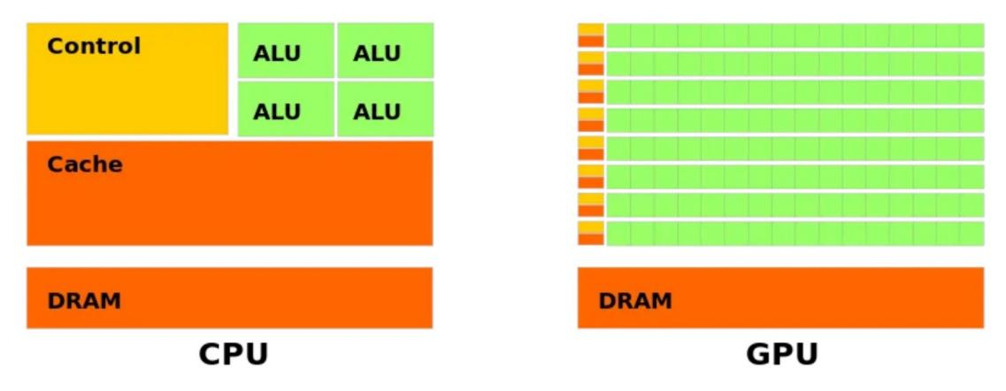
Left: CPU architecture; right: GPU architecture. Source: https://www.omnisci.com/technical-glossary/cpu-vs-
