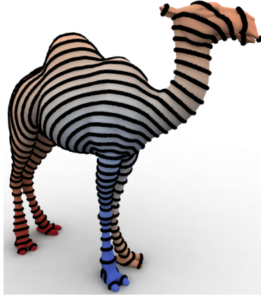
Figure 7: Level sets of geodesic distance to the front right toe of a 3D camel model approximated using the optimal transport technique [SRGB14a].
