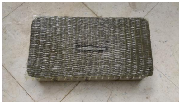
Figure 6: FRPP4, FRP-bonded concrete panel, angled 3" x 0.25" defect
