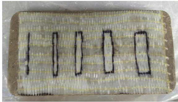
Figure 5: FRPP5, FRP-bonded concrete panel with multiple defects
