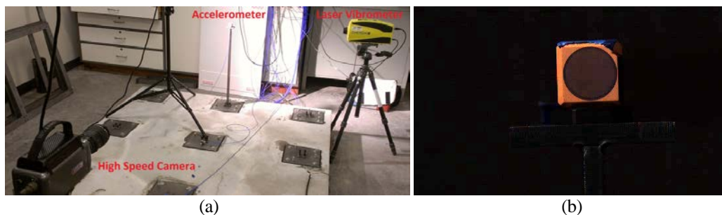
Figure 1: (a) Labeled picture of experimental setup and (b) screenshot of scene from camera (artificially brightened for visibility) [3]
