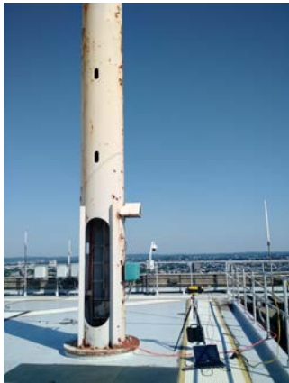
(a) Laser vibrometer measurement setup (b) Measurement result with static reference for comparison Figure 3 Laser vibrometer verification of MIT Green Building crow's nest resonant frequency
