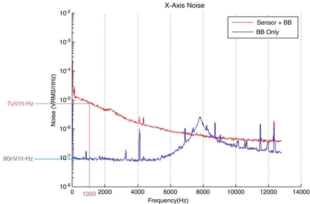
**Fig. 26.5** Breadboard front end X-axis noise. *BB*: breadboard
