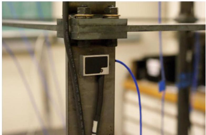
largest laboratory structure configuration planned, the network had to accommodate up to 120 triaxial accelerometers. To measure the propagation of waves through the structure, accelerometer outputs were synchronized to within 0.1 ms. Lastly, the MIT CEE team established the requirement to monitor structural modes up to 1 kHz necessitating a sampling rate of at least 2 kHz per channel. These requirements are summarized in Table 26.1.
