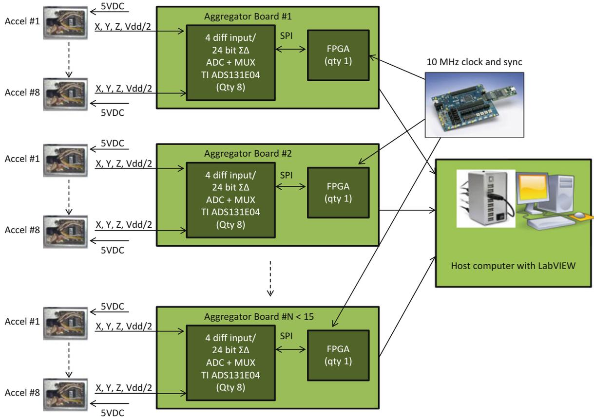
**Fig. 26.3** Modular architecture for accelerometer network. Each aggregator board accommodates eight accelerometers and can be added to grow the size of the network. Single clock for data synchronization is also shown
