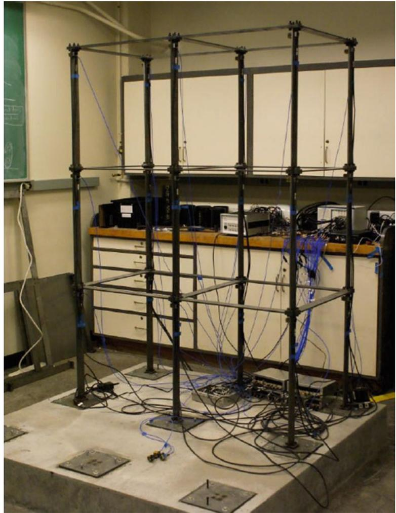
**Fig. 26.2** Draper accelerometer assembly installed on lab structure
