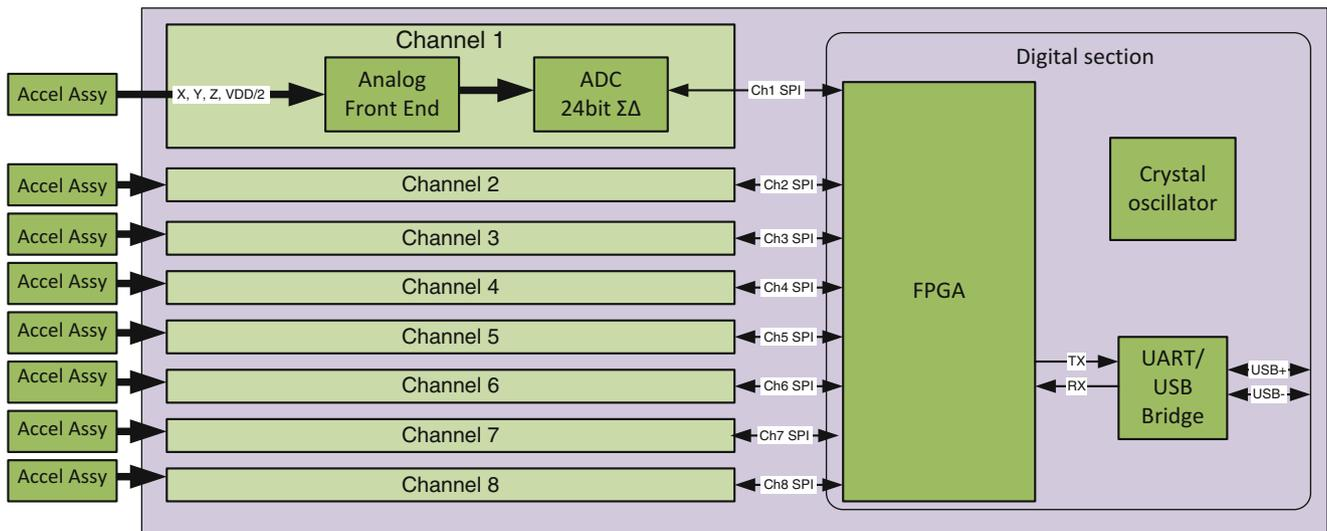
**Fig. 26.4** MITEI aggregator board functional block diagram
