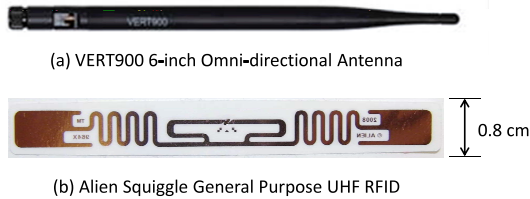
Figure 9—Antenna and commercial UHF RFID used in experiments: (a) We move the VERT900 6-inch vertical antenna in a straight line to emulate a linear antenna array. (b) the Alien Squiggle General Purpose UHF RFID Tags. The sizes of (a) and (b) are not proportional to the real sizes of the devices.
