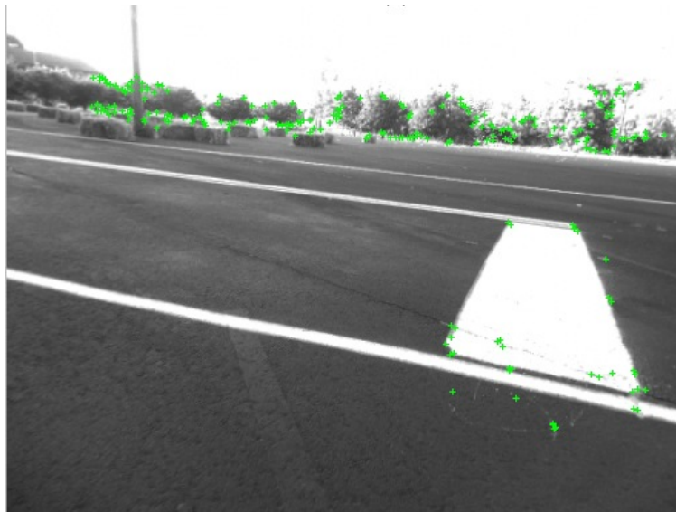
(b) Another example where a ground surface with low texture results in degenerate data.
