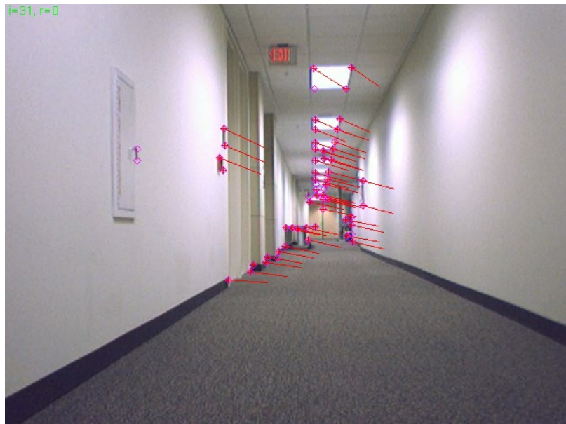
(b) Camera image with measurements and reprojected structure.
