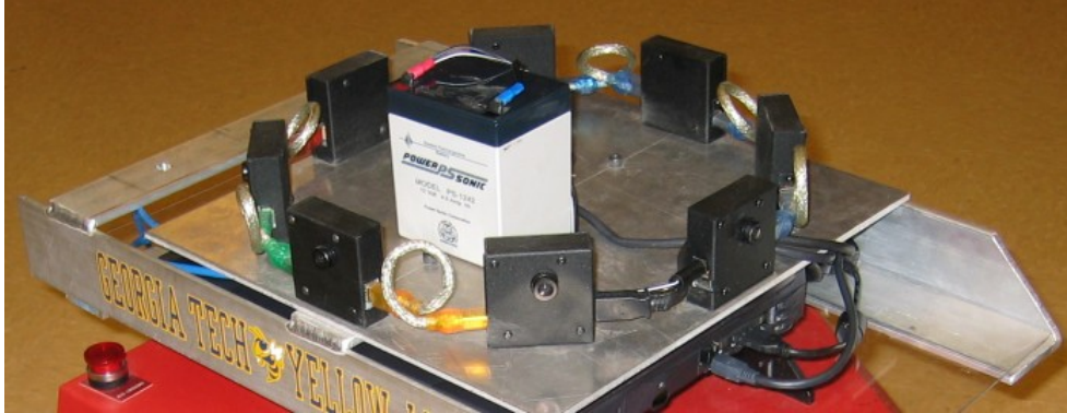
Figure 6: Custom made camera rig, mounted on top of an ATRV-Mini mobile robot. Eight Fire-Wire cameras are distributed equally along a circle and connected to an on-board laptop.
