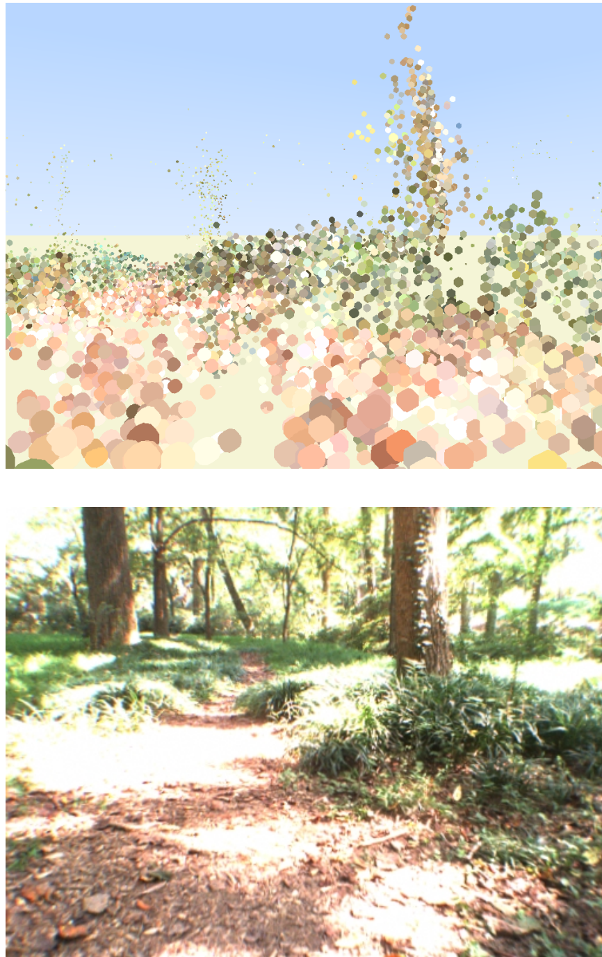
Figure 47: Batch 3D point cloud reconstruction based on the feature tracks provided by visual odometry. Every frame and all successfully tracked features from visual odometry were used, resulting in longer computation times. Each sphere corresponds to one feature, which is colored based on the corresponding pixels in the input images. All spheres have the same size, so that their reprojected size is due to perspective effects. A robot camera image from a similar view point is shown for reference.
