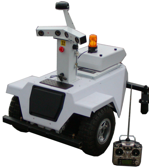
Figure 42: The DARPA LAGR mobile robot platform with two front-facing stereo camera rigs, a GPS receiver as well as wheel encoders and an inertial measurement unit (IMU).
