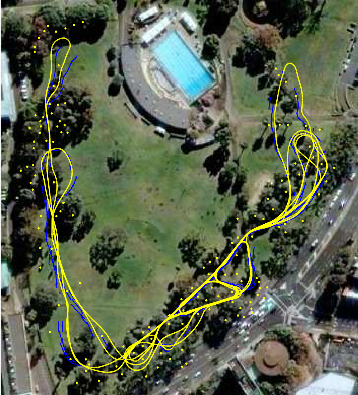
Figure 17: Results for the full Victoria Park sequence. Solving the complete problem including data association in each step took 3.4 minutes on a laptop computer. Since the dataset is from a 26 minute long robot run, iSAM is over 7 times faster than real-time in this case, calculating the complete and exact solution for each of the almost 7000 steps. The trajectory and landmarks are shown in yellow (light), manually overlaid on an aerial image for reference. Differential GPS was not used in obtaining my experimental results, but is shown in blue (dark) for comparison - note that in many places GPS was not available, presumably due to obstruction by trees.
