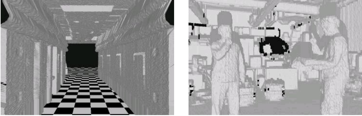
Figure 2: An example of 3D laser-based mapping [76] without SLAM. Note that the 3D model of the hallway curves to the left because of accumulated error from robot odometry.
