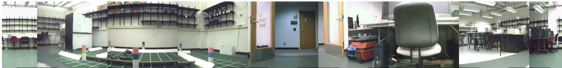
Figure 7: Combined snapshot from all eight cameras, providing a 360^\circ view. Note that the images do not fit perfectly as the cameras have different optical centers.
