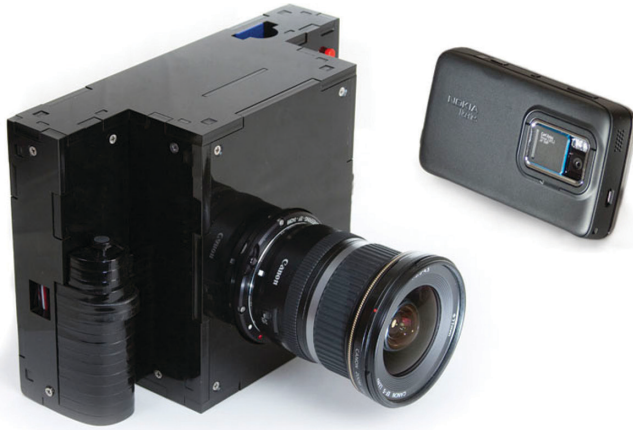
Figure 1. Two implementations of the Frankencamera architecture: The custom-built F2 (left)—portable and self-powered, best for projects requiring flexible hardware; and the Nokia N900 (right) with a modified software stack—a compact commodity platform best for rapid development and deployment of applications to a large audience.
