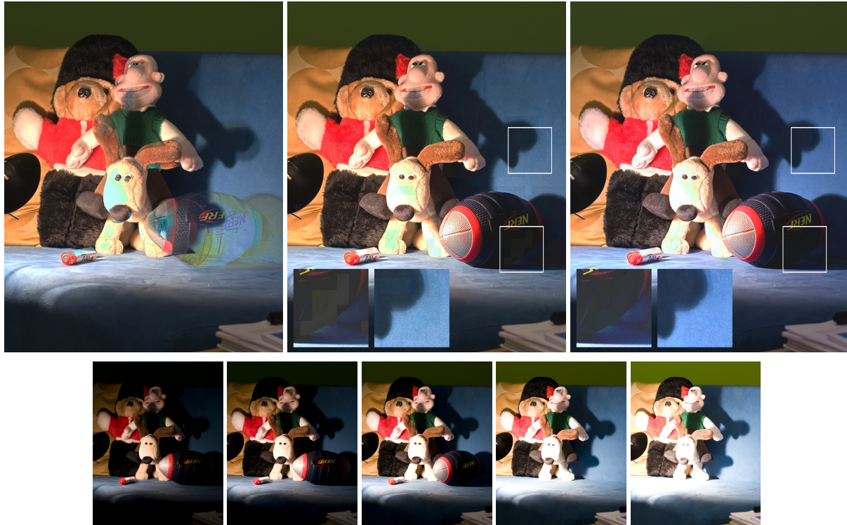
Figure 3. First row from left to right: simple HDR image with ghosting, the output of our algorithm before blending, and our result after blending. Particularly in smooth areas, abrupt changes at the boundary of different patches are visible before blending. The second row shows the original exposures in the stack (note that the scene changes substantially with some objects moving and some disappearing).
