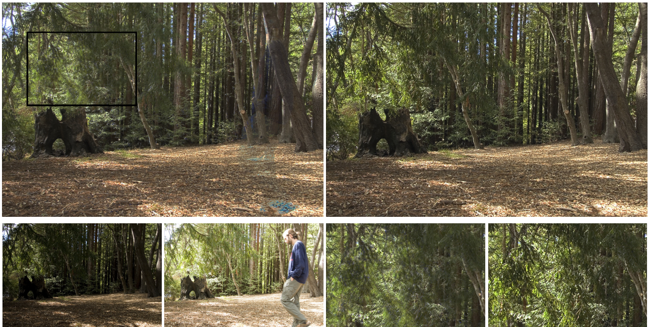
Figure 4. The top left image is the simple HDR image with ghosting from a sequence of 4 pictures taken in a forest. A person walking in the scene causes ghosting on the right side of the left image. Moreover, the branches present strong artifacts due to the wind blowing. The top right image is our result. A detail from standard HDR and our result can be seen in the bottom row (right), together with two images from the stack (left).
