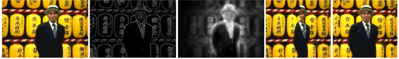
Figure 3. The importance map directly influences the retargeting result. From left to right: input image, gradient-based and context-aware 6 importance maps, and outputs from seam carving using the gradient-based and the context-aware maps. Adapted from Goferman et al. (2010) 6 (©2010 IEEE).
