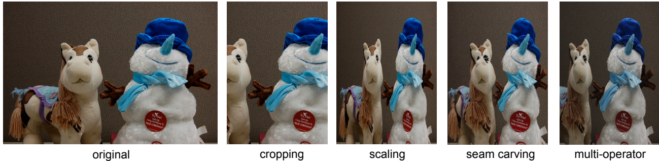
Figure 9. Individual retargeting operators have advantages and disadvantages, and combining multiple operators can lead to better results. The original image is retargeted using cropping, scaling, seam carving, and a combination of cropping, seam carving, and scaling.
