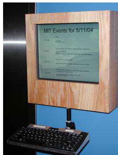
Figure 1: The OK-net terminal with a touch panel display and an optional keyboard.
