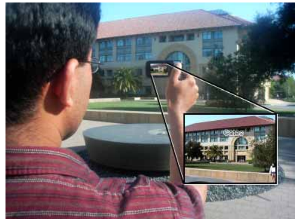
Figure 1: A snapshot of the outdoors augmented reality system being used. The system augments the viewfinder with information about the objects it recognizes in the image taken with a phone camera.
