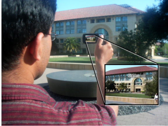
Figure 1. Our outdoors augmented reality system augments the viewfinder with information about the objects it recognizes in the image taken with a phone camera.
