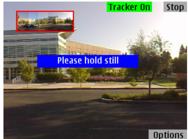
Figure 5. Panorama is automatically captured and constructed as user pans the camera around the scene.
