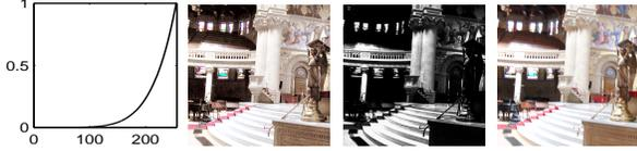
**Fig. 3.** Color weighting: weight function, short-exposed image, weight image, and a long-exposed image.
