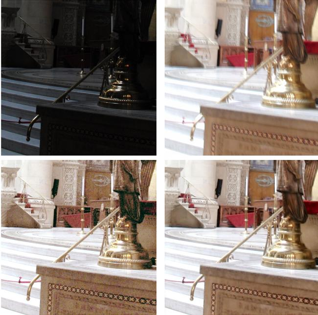
**Fig. 5.** Image enhancement result: short- and long-exposed images (upper row), the photometrically calibrated short-exposed image (bottom left), and the result (bottom right).
