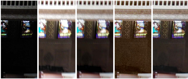
Fig. 6. Solving under-exposed areas in shortest exposed image. From left to right: two input images, the exposure fusion result, the photometrically calibrated shortest exposure (i.e., noisy image), and our result.
