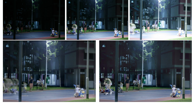
Fig. 3. Example with ghosting artifacts in addition to blur caused by camera shake blur: exposure fusion (second row left), and our result (second row right). Both results have been obtained by fusing the three images (top).
