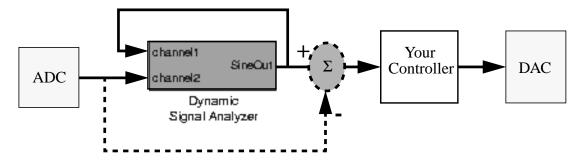
Figure A.2: Linking Additional Components with the DSA Block
