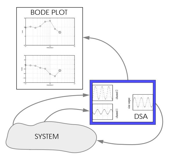
Figure 1.1: DSA and a System to be Analyzed
