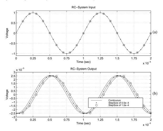
Figure 5.3: Discrete Sampling Lag with 1kHz Sine Wave
