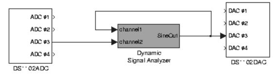
Figure A.1: Dynamic Signal Analyzer Measuring System Response
