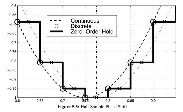
Figure 5.5 shows an enlarged section of the previous figure. The sampling interval here creates a stepping pattern that is symmetric about the vertical line at x = 0.775, as shown above. Because of the symmetry, it is clear the phase of the predominant harmonic component (i.e. the original, continuous frequency) is shifted by exactly half a
