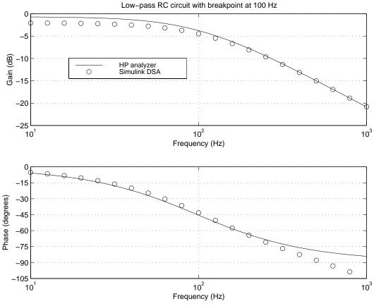
Figure 5.1: Low-Pass RC Cicuit Response
