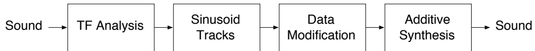
Figure 3.3: The McAulay-Quatieri analysis/synthesis system extends the phase vocoder by extracting sinusoid tracks from the time-frequency analysis data.
