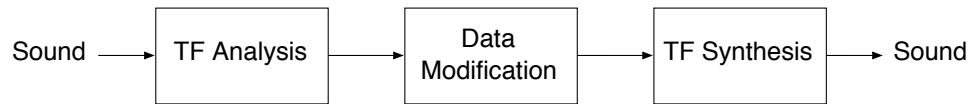
Figure 3.1: The phase vocoder analyzes a sound, modifies the analysis data, and synthesizes the sound.
