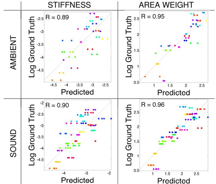
Figure 4: Comparisons between ground truth and model predictions on material properties estimated from videos of fabric excited by ambient forces and acoustic waves. Each circle in the plots represents the estimated properties from a single video. Identical colors correspond to the same fabric. The Pearson product-moment correlation coefficient (R-value) averaged across video samples containing the same fabric is displayed.
