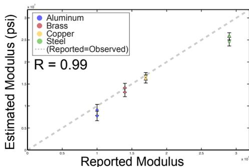
Figure 3: Estimating the elastic modulus of clamped rods: Young’s moduli reported by the manufacturer are plotted against values estimated using our technique for aluminum, brass, copper, and steel. Estimated values are close to those reported by the manufacturer.
