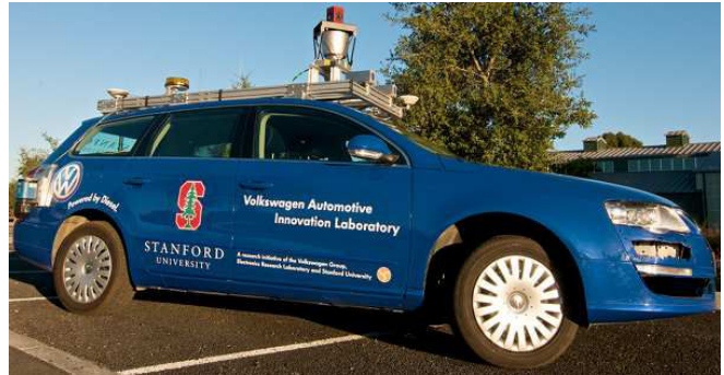
Fig. 1. Junior: Stanford’s autonomous research vehicle.
