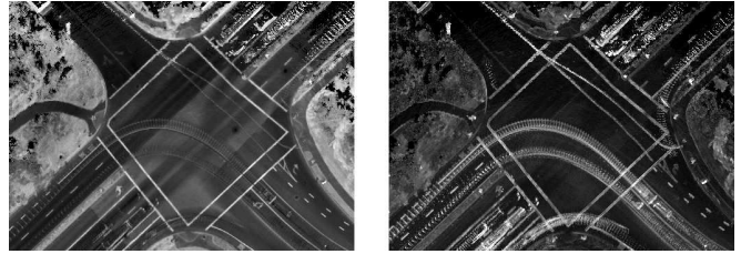
Fig. 3. The two channels of our probabilistic maps. On the left we see the average infrared reflectivity, or brightness, of each cell. Our approach is novel in also considering the extent to which the brightness of each cell varies, as shown on the right.
