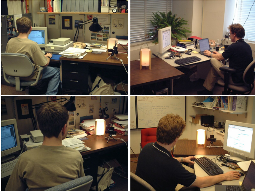
Fig. 5. The two upper images show the level of physical presence when both users are in their office but not explicitly looking at the lamp (which is dim). In the lower images, one of the users has noticed his lamp getting brighter and has returned that gaze.
