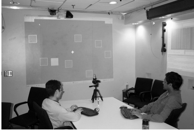
Fig. 3. Setup for the room experiment. The SRI stereo camera is placed on the table.
