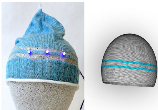
Fig. 17. Conductive yarn (cyan faces) can be integrated into the body of the object for incorporating electronics.
