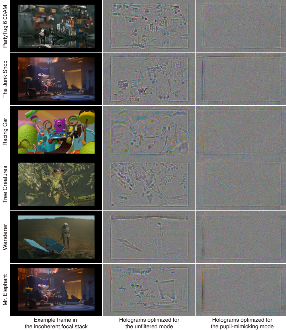
Fig. S16. Visualization of exemplary focal stack images and holograms optimized for unfiltered and pupil-mimicking modes for scenes used in this paper.
