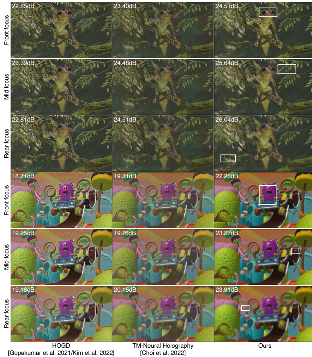
Fig. S8. Additional experimental results captured in the unfiltered mode. The captured results are presented in 900 DPI resolution for close-up examination. Source image: “Tree Creature” by Daniel Bystedt, and “Racing Car” by Pokedstudio. The “Tree Creature” shows recording planes 9, 17, 28, the “Racing Car” shows recording planes 5, 15, 27.
