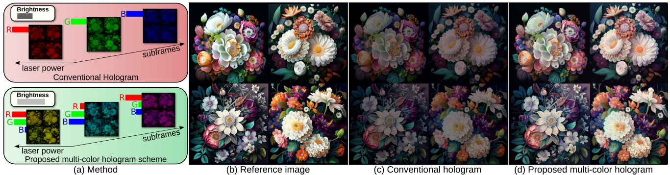
Fig. 1. Our framework simultaneously uses multiple laser light sources to support brighter images in holographic displays. (a) Conventional holograms display full-color images using single-color holograms, each dedicated to a color channel and illuminated by a single laser light source. Our method instead optimizes multi-color holograms, each lit by and modulates multiple laser light sources. Given a reference image (b), photographs captured from a holographic display prototype with an 80 ms exposure: (c) A conventional hologram reconstructs an image with limited brightness, and (d) A multi-color hologram reconstructs a brighter image (Source image: Midjourney, Link: Github:complight/image ).
