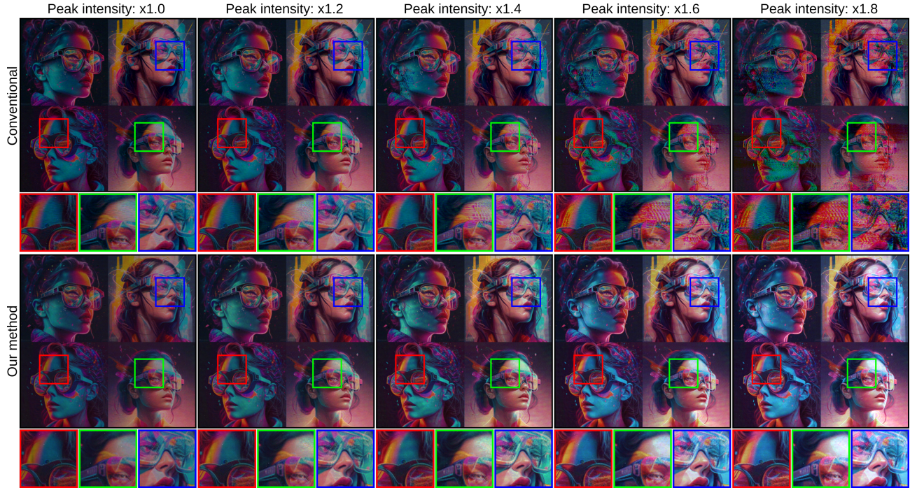
Fig. 3. Increasing peak intensity levels with our multi-color hologram scheme. Photographs show that our method can enhance the peak intensity levels of the captures up to \times 1.8 without noticeable artifacts or distortions. In contrast, the conventional hologram fails to support beyond \times 1.0 (Source image: Midjourney, Link: Github:compliant/image , 140 ms exposure).
