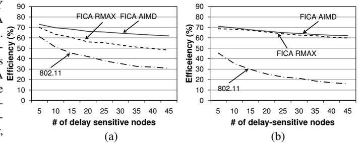
**Figure 10: Mixed traffic. Five nodes are fully saturated. All other nodes have delay-sensitive traffic with a uniform distribution between 800Kbps to 5Mbps. (a) 802.11 PHY 150Mbps; FICA 145Mbps. (b) 802.11 PHY 600Mbps; FICA 580Mbps.**
