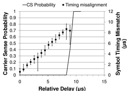
**Figure 13: CDF of timing misalignment with carrier sensing. The dark line shows the carrier-sensing probability and the rectangular points show the measured symbol timing difference.**
