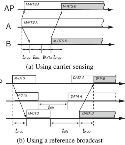
**Figure 6: The worst-case symbol timing misalignment of two concurrent transmissions received at the AP in a CSMA WLAN: (a) symbol timing misalignment when coordination uses carrier sensing; (b) a reference broadcast synchronizes the senders better and timing misalignment is much tighter.**
