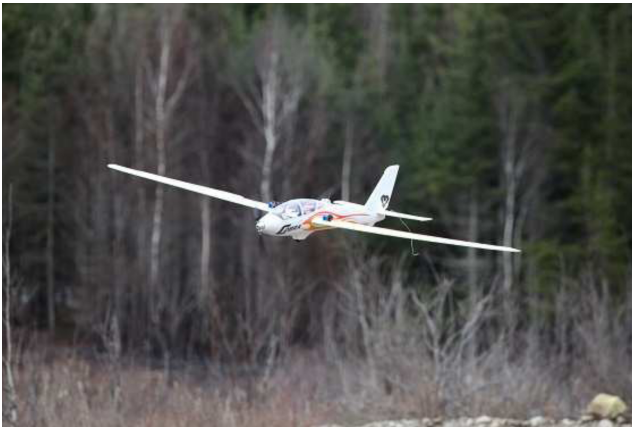
Fig. 1. University of New Brunswick collaboration based robotics and automation (COBRA) group fixed-wing powered glider with a 2.4 meter wing span that was used for experimental validation of the proposed area coverage algorithm (photo courtesy Yvon Thibault).
