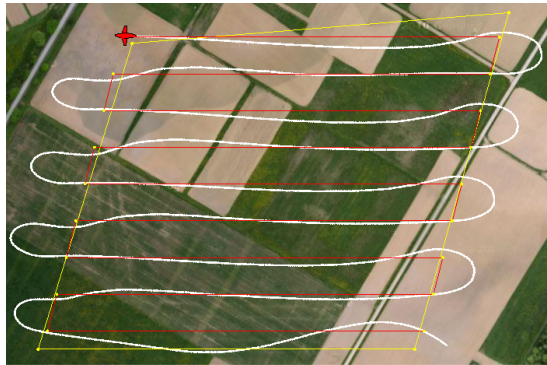
Fig. 12. Path taken to cover workspace using preplanned lawn mower path in HWIL simulation.
