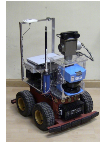
Fig. 8. The ASys robot control testbed includes construction of self-aware robot controllers [37] for mobile robot applications. The figure shows the Higgs robot, the main platform for this research [36].
