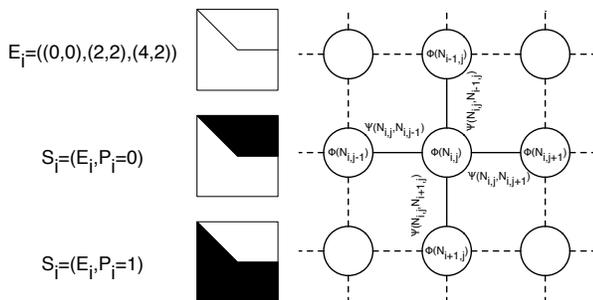
Figure 1: Left: An example edge assignment and the two possible segmentation assignments it can create depending on its parity. Right: A section of a Markov random field.
