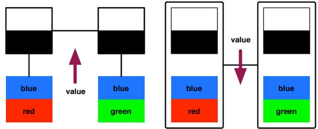
Figure 2: Left: A traditional MRF might give a high value to this pairing of horizontal edges, since each image patch gives strong local evidence and the edges continue each other. Right: An MRF that combines the edge and image variables into the same nodes can give a low value to this combination because it is creating a segment with differently colored neighboring pixels.
