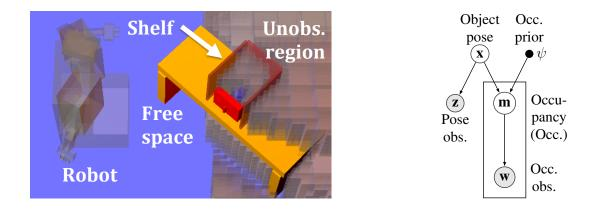
**Figure 5-1:** A mobile robot uses object detections to infer regions of occupied space, and uses free space observations to eliminate possible locations of objects. The framework in this chapter allows inference across representational layers as depicted by the graphical model; see Sections 5.1–5.3 for details.
