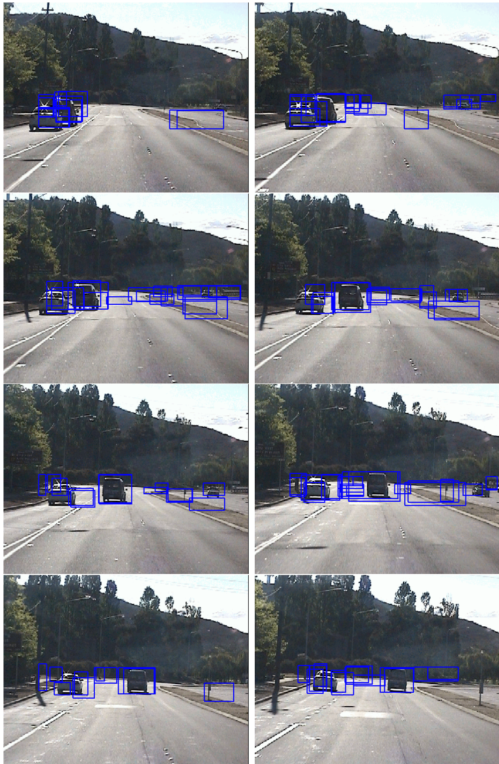
Figure 4.28: Detected obstacle candidates in two vehicle sequence. The video of this sequence is in the Appendix DVD-ROM (Page 257 )
