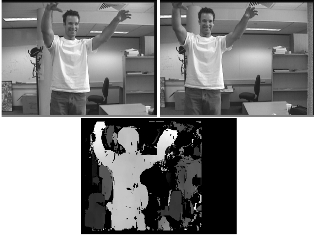
Figure 4.13: top: Typical stereo images from people tracking experiment bottom: estimated disparity
