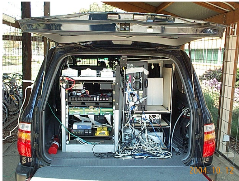
Figure A.13: Back of vehicle featuring desktop computers, networking, relay and breakout racks.
