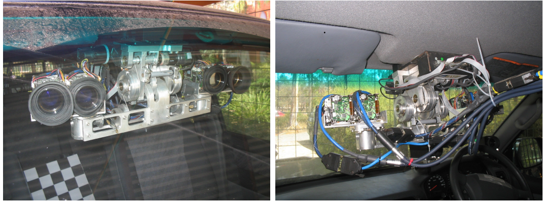
Figure A.6: CeDAR: Cable Drive Active vision Robot in vehicle. Four cameras are arranged in two stereo pairs. Cameras are fitted with polarising filters and far field cameras use glare hoods.
