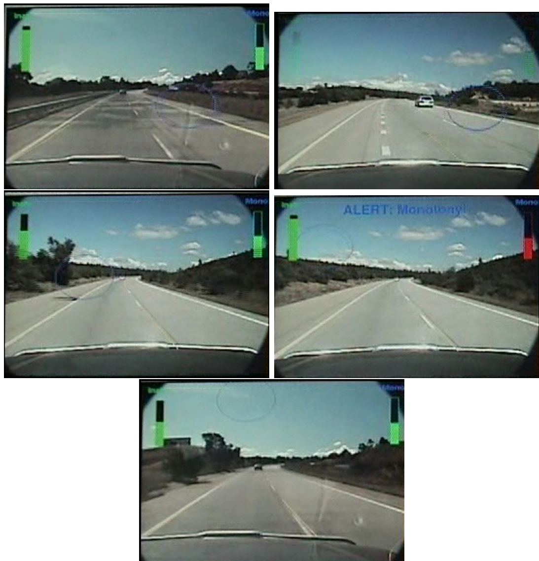
Figure 7.32: Sequence of screen-shots of the Automated Co-driver showing a Monotony warning occurring. Large circles: driver gaze.
