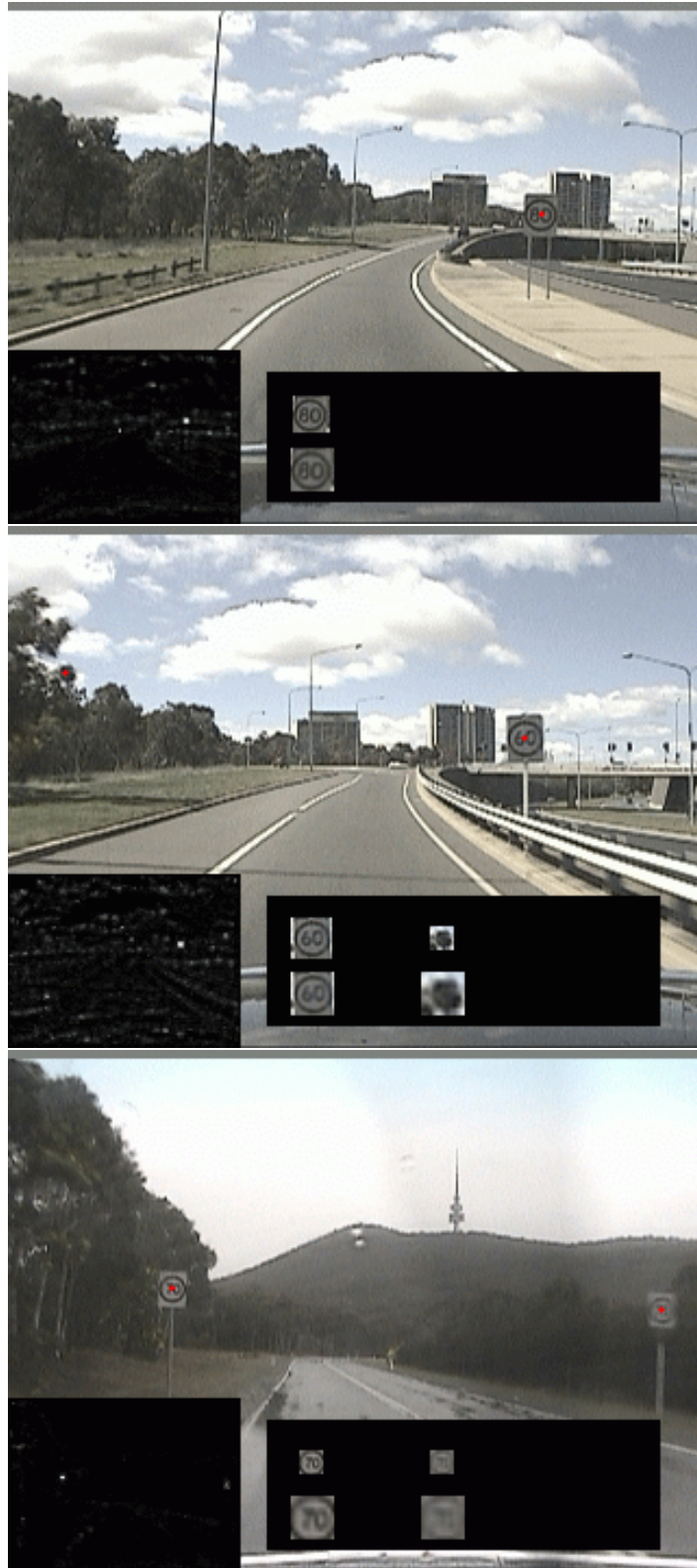
Figure 5.4: Speed sign detection using Fast Radial Symmetry Transform. Bottom left corner shows FRST image, The red crosses highlight detected signs.
