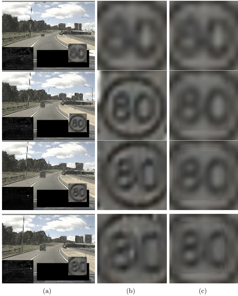
Figure 5.16: ‘80’ sign enhancement. (a) : Every 10th frame from Sixty sequence. (b) : Resized cropped original image. (c) : Enhanced sign image.
