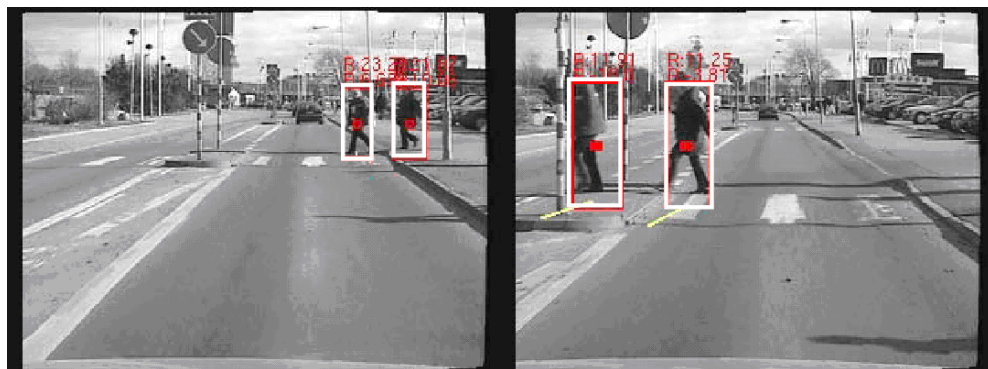
Figure 7.19: Online pedestrian detection. The basis for the system used in the Automated Co-driver.
