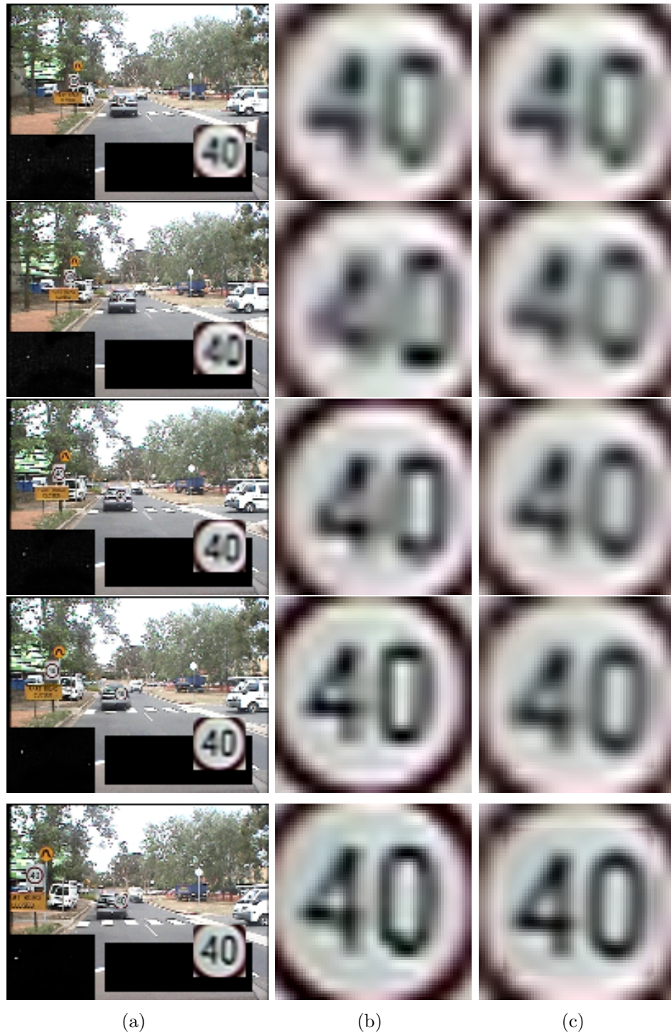
Figure 5.14: ‘40’ sign enhancement. (a): Every 10th frame from Forty sequence. (b): Resized cropped original image. (c): Enhanced sign image.
