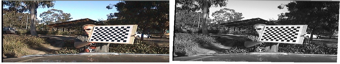
Figure A.8: Left wide field camera before and after image rectification.
