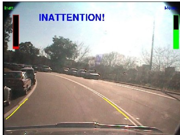
Figure 7.26: Screen-shots of the Automated Co-driver. Prolonged inattention detected. Large circles : driver gaze.
