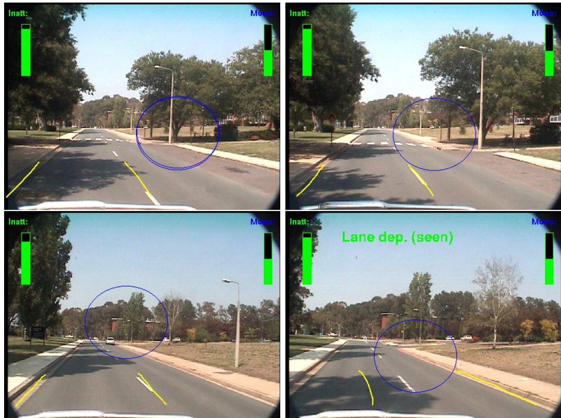
Figure 7.28: A sequence of Screen-shots of the Automated Co-driver. A lane departure that was seen by the driver is shown. Large circles: driver gaze.
