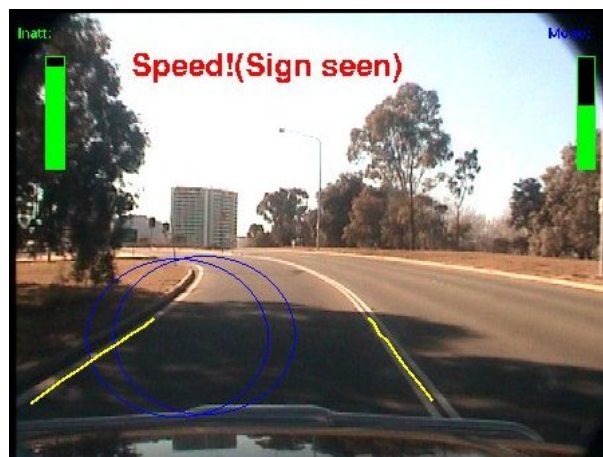
Figure 7.26: Screen-shots of the Automated Co-driver. Prolonged inattention detected. Large circles : driver gaze.
