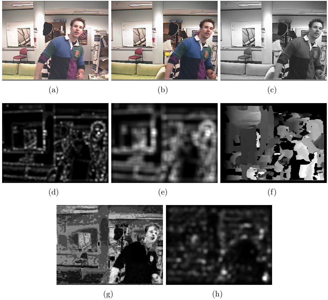
Figure 3.10: Preprocessing a colour stereo image pair. (a) Image from camera 1, (b) Image from camera 2, (c) Intensity image, (d) Radial symmetry image, (e) Facial symmetry image, (f) Depth map, (g) Skin colour likelihood image, (h) Radial symmetry of skin colour likelihood image searching for a radius of 15 pixels.
