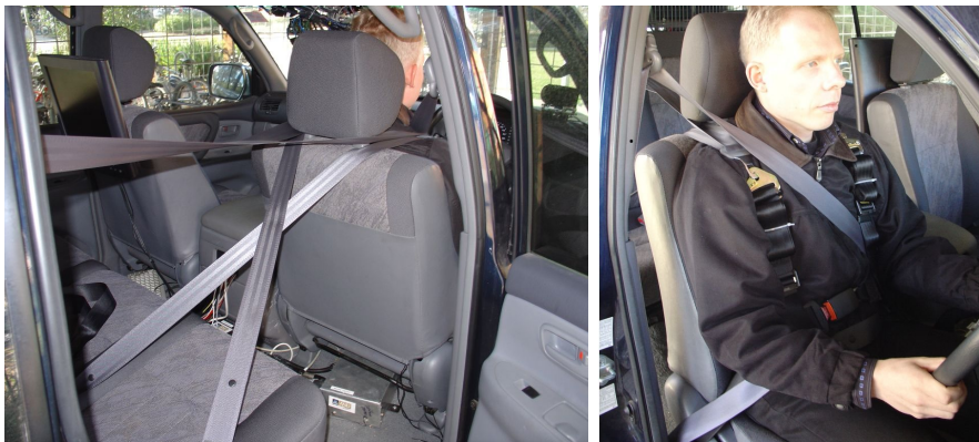
Figure A.12: Driver wearing 4-point safety harness. Rear seat belts fully extended and crossed for use as top harness straps.
