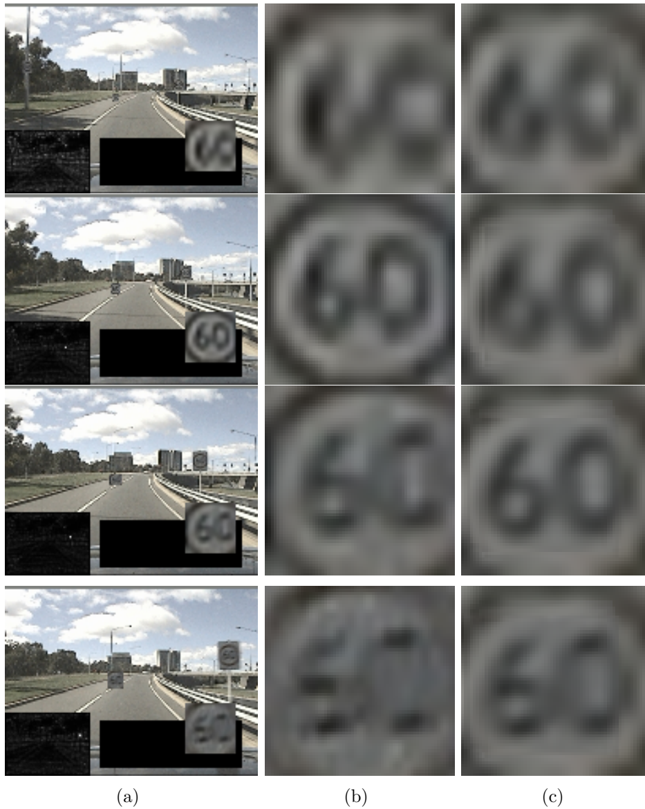
Figure 5.15: ‘60’ sign enhancement. (a) : Every 10th frame from Sixty sequence. (b) : Resized cropped original image. (c) : Enhanced sign image.
