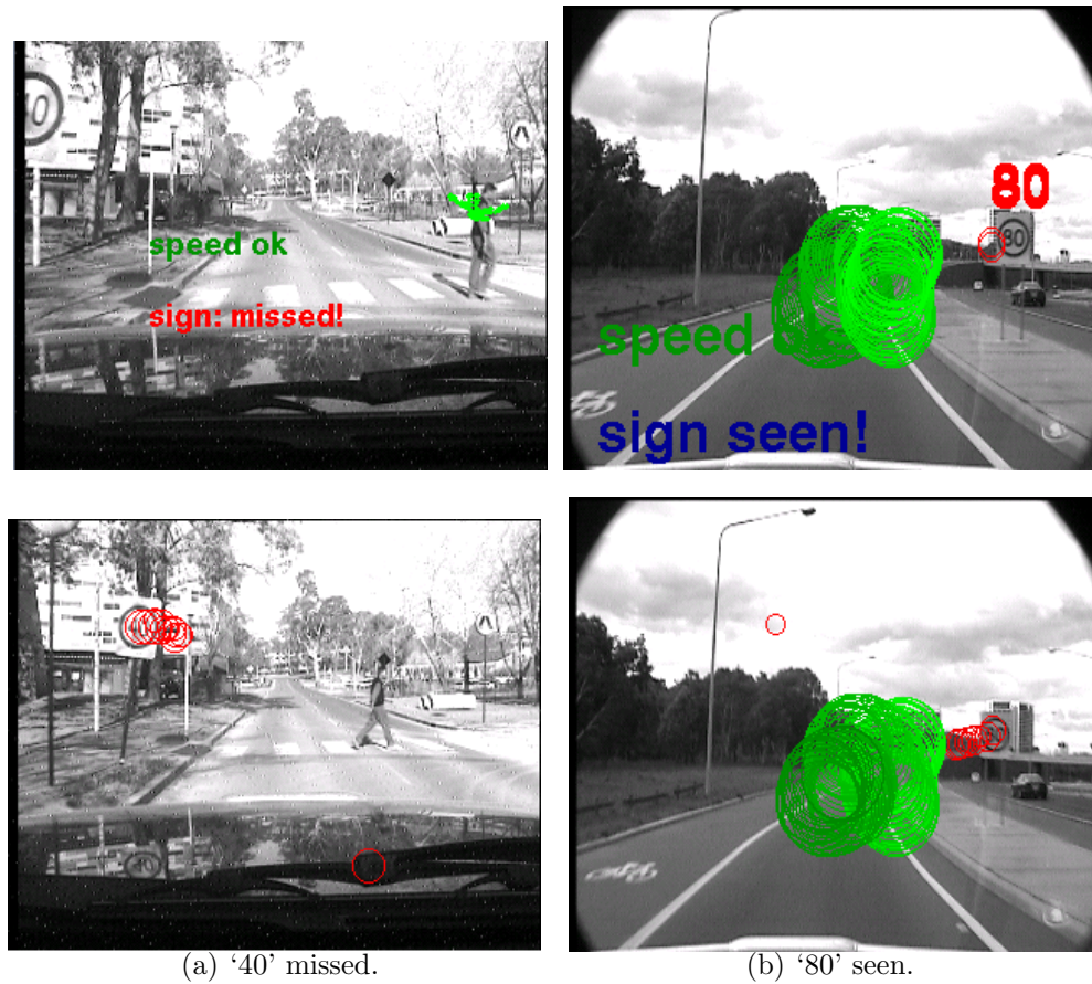
Figure 7.11: Primary scenarios for Road Signs Automated Co-driver when the vehicle is speeding. left: Live video feed showing current view, eye gaze ( dots / large circles ) and current status ( overlaid text ) during screen-shot. right: Last detected sign ( small circles ) and eye gaze ( dots / large circles ).
