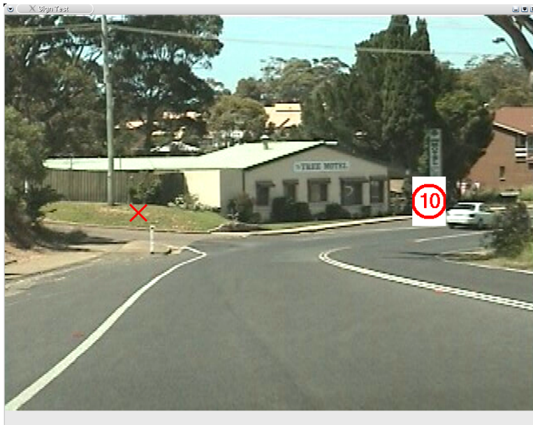
Figure 7.3: Screen-shot of PC test application to gather data on gaze object recognition field of view. A test subject is requested to fix gaze on the cross. The Speed sign periodically varies in position and speed (10,20,30,...,90). A road video sequence was played in the background to add context for the trials. The subject entered the ‘guessed’ sign via numeric keypad (‘1’-‘9’).
