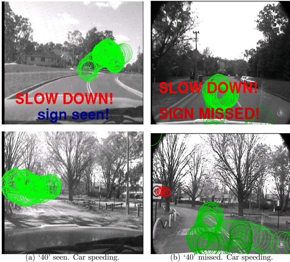
Figure 7.12: Primary scenarios for Road Sign Automated Co-driver when the vehicle not speeding. left: Live video feed showing current view, eye gaze ( dots / large circles ) and current status ( overlaid text ) during screen-shot. right: Last detected sign ( small circles ) and eye gaze ( dots / large circles ).
