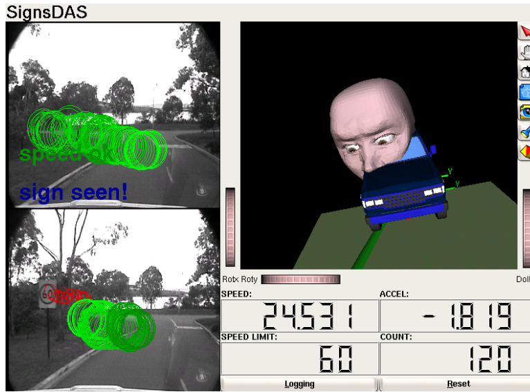
Figure 7.10: Screen-shot showing ‘60’ sign detected and seen by driver. top left: Live video showing eye gaze ( large circles ) and status ( overlaid text ). bottom left: Last detected sign ( small circles ) and eye gaze ( large circles ). top right: 3D model of current vehicle position, eye gaze ( oversize head ) and sign location. bottom right: Current detected speed limit, vehicle speed, acceleration and count down for speeding grace period in frames.
