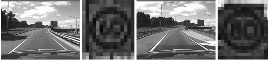
Fig. 9. Still frames from a video camera, with close ups of speed sign. Classifying the signs as 60 or 80 is not obvious.
