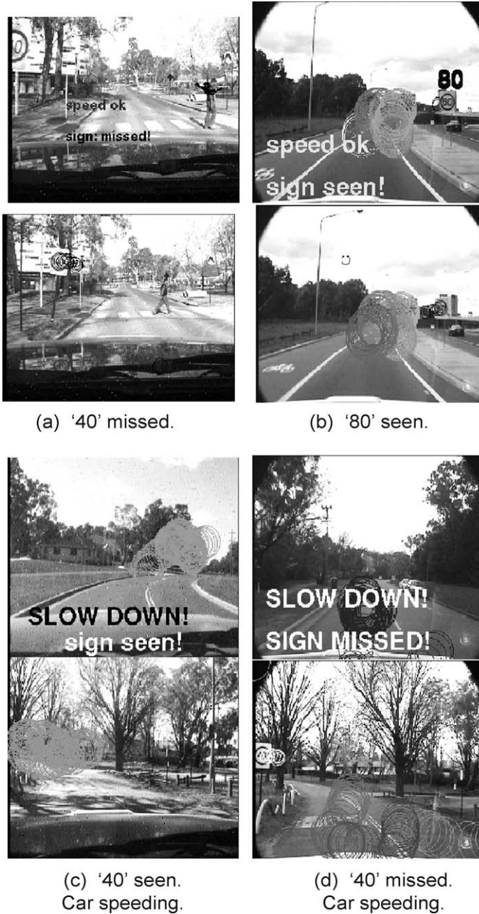
Fig. 8. Primary scenarios for signs driver assistance system. Left: live video feed showing current view, eye gaze (dots/large circles) and current status (overlaid text) during screenshot. Right: last detected sign (small circles) and eye gaze (dots/large circles).
