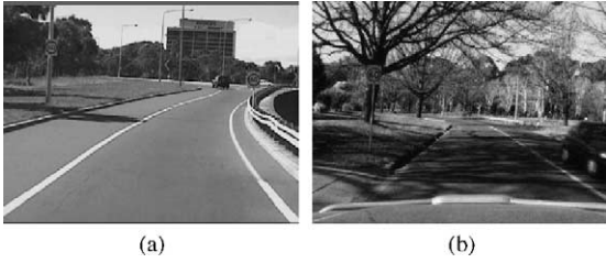
Fig. 2. (a) Algorithms assuming strong road scene structure can miss valuable information, such as a sign on an unexpected side of a lane. (b) Assuming common regions such as sky and road can be identified by large areas of self-similar colour is not always valid.
