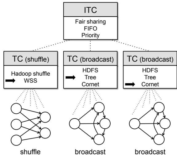
**Figure 4: Orchestra architecture. An Inter-Transfer Controller (ITC) manages Transfer Controllers (TCs) for the active transfers. Each TC can choose among multiple transfer mechanisms depending on data size, number of nodes, and other factors. The ITC performs inter-transfer scheduling.**
