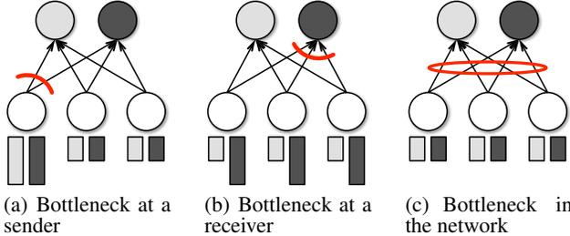
**Figure 6: Different bottlenecks dictating shuffle performance.**
