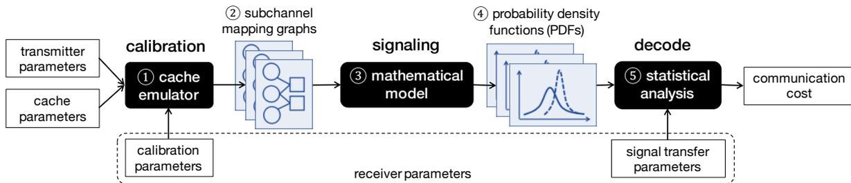
Fig. 6: CaSA: end-to-end quantitative security analysis framework.
