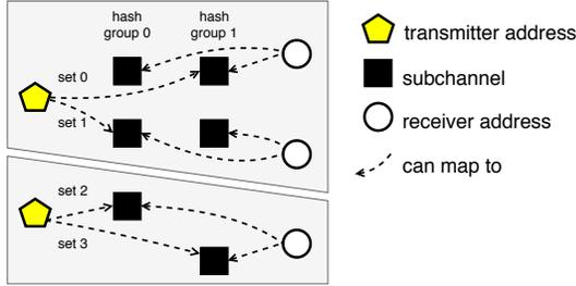
Fig. 7: An example of subchannel mapping graph.
