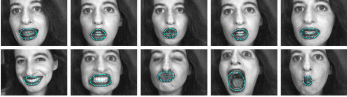
Figure 2.3 – Automatically tracking mouth positions of test subject in a video stream. Lip positions are found via a deformable template and fit to an ellipse using least squares. The upper images contains excerpts from speech segments, corresponding left to right with phonemes: /eh/, /ae/, /uw/, /ah/, and /iy/. The bottom row contains non-speech mouth positions. Notice that fitting the mouth to an ellipse can be non-optimal, as is the case with the two left-most images; independently fitting the upper and lower lip curves to low-order polynomials would yield a better fit. For the purposes of this example, however, ellipses provide an adequate, distance invariant, and low-dimensional model. The author is indebted to his wife for having lips that were computationally easy to detect.
