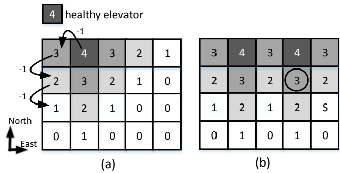
Fig. 4. Elevator index sharing in the northward virtual network for (a) one and (b) two healthy elevators assuming an initial index value of 4.
