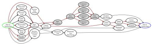
Fig. 3. Task-graph of the wind turbine system application.
