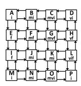
(a) A generic 2D-mesh heterogeneous multi-cores.
