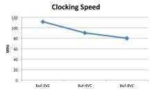
Fig. 7. Effect of virtual channels on router clocking speed.
