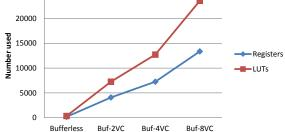
Fig. 6. FPGA resource utilization per router configuration.
