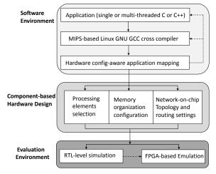
Fig. 1. Heracles-based design flow.
