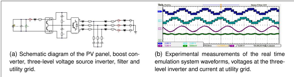
**Figure 5:** Utility Grid Connected Photovoltaic Converter System Application.
