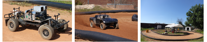
Fig. 1: (left) The AutoRally car: weight 22 kg; LWH 1m×0.6m×0.4m. (middle) High-speed off-road driving task. (right) Test track
