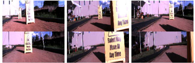
Fig. 3: Real obstacle avoidance task: onboard camera images showing the car avoiding two obstacles successively.
