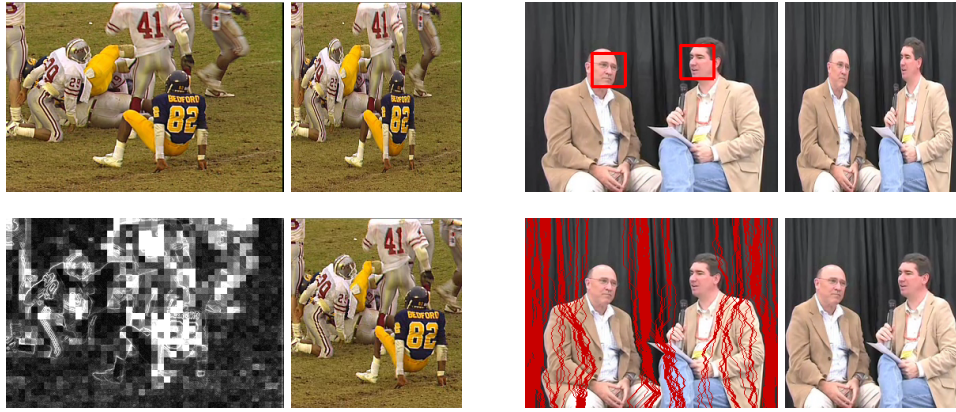
Figure 1.14: Retargeting using external energy (saliency) functions. On the left, from left to right and top to bottom: a frame from the football video; saliency map used by [48]; the rescaled frame; the retargeted frame. On the right, in the same order: a frame from the interview video, with the detected face regions; the calculated seams for this frame, accounting for the faces constraints; the rescaled frame; the retargeted result.
