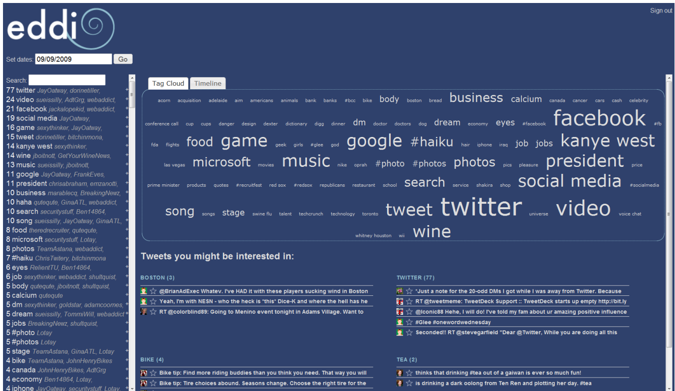
Figure 1. Eddi is a topic-oriented browsing interface for Twitter. Clockwise from upper right is the tag cloud, timeline (hidden in another tab), the topic dashboard, and the navigational list.
