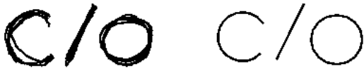
Figure 25: Examples of overtracing. Overtraced objects on the left, system’s output on the right.
