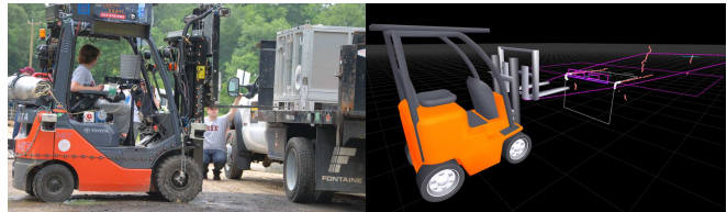
Fig. 1. The prototype forklift that is the host platform for the mobile manipulation algorithm presented in the paper. The vehicle autonomously detects and engages unknown pallets, picking them up from, and placing them onto the ground or the bed of a truck. The rendering on the right depicts the corresponding output of the pallet and truck estimation algorithms.
