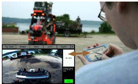
Fig. 2. Forklift being commanded via the tablet PC to pick up a pallet that is stationed on a truck bed.
