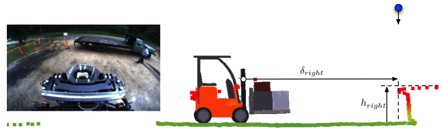
Fig. 6. Truck bed detection algorithm depicted with raw data (false-colored by height) acquired from the sensor mounted on the right of the mast.
