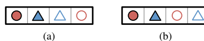
Fig. 1. Benefits of task permutation. Filled shapes are robots, unfilled shapes are goal configurations, and the black shape represents the boundary. While both are optimal task assignments, (a) is infeasible but (b) is feasible.
