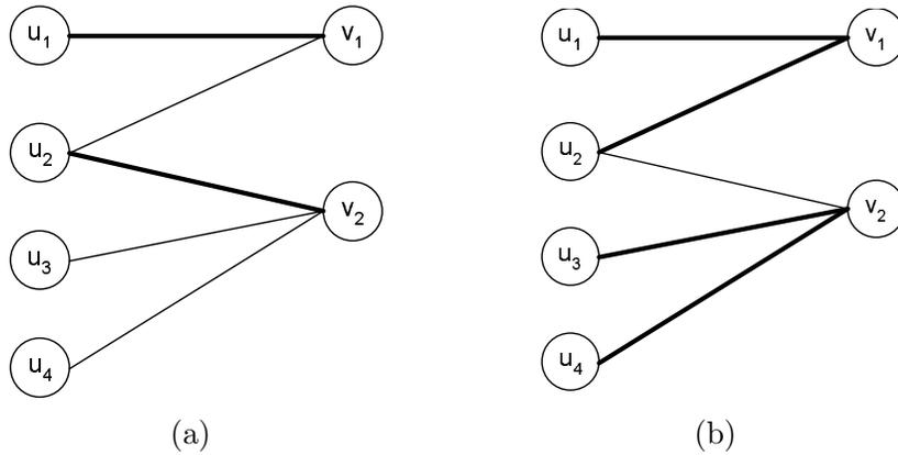
Fig. C.1. The maximum matching in (a) cannot be extended to the unique optimal semi-matching, shown in (b).
