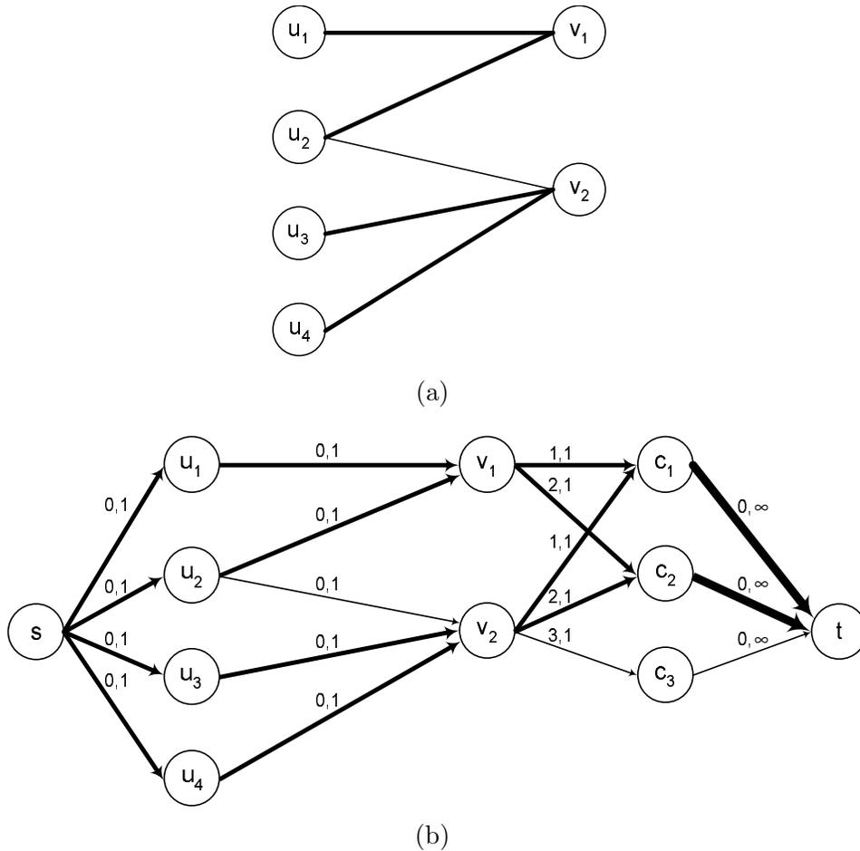
Fig. 1. (a) shows a graph in which the bold edges form an optimal semi-matching. (b) shows the corresponding min-cost max-flow problem. Each edge is labeled with two numbers: a cost, and a capacity constraint. Bold edges carry one unit of flow and doubly-bold edges carry two units of flow in  $G$ .
