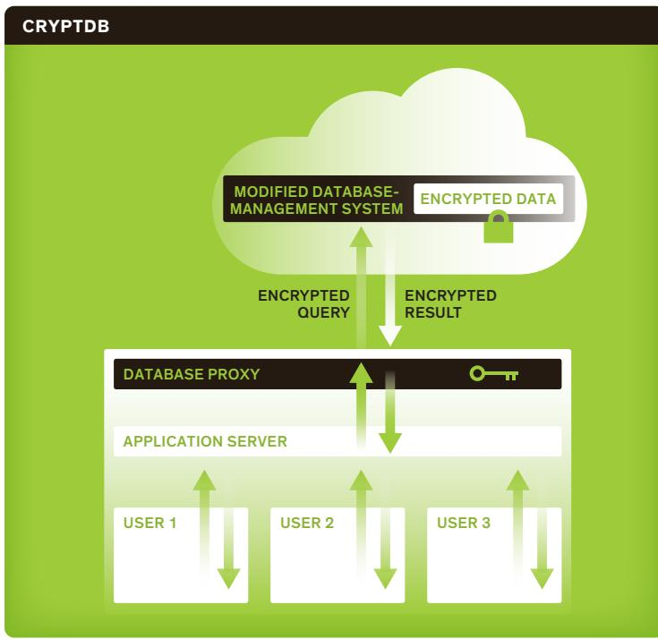
**SECURITY IS OFTEN** a concern when information is held in a cloud database. CryptDB addresses this issue by encrypting the data in a way that still allows normal database queries to be performed. The application itself runs locally, as does a database proxy, which performs the encryption and decryption. The proxy also translates queries into a form that can be run on the modified database-management system running in the cloud.
