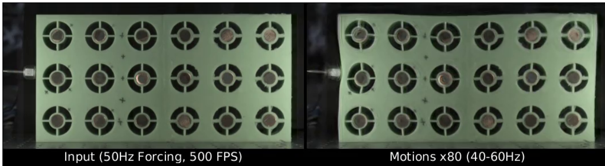
Movie S4. A probe vibrates the metamaterial at 50Hz. The input high speed video is shown on the left. Motions within a 40-60 Hz frequency band are amplified 80 times to produce the video on the right, in which the propagation of the vibrations is revealed. The video was recorded at 500 FPS and is played back at 30 FPS.
