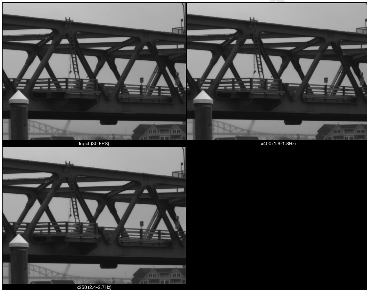
Movie S2. The input bridge video is concatenated with two motion magnified videos revealing different modal shapes of the bridge. Motions within a 1.6-1.8 Hz frequency band are amplified 400 times to produce the video on the right, in which the first bending mode is revealed. Motions within a 2.4-2.7 Hz frequency band are amplified 250 times to produce the video on the bottom, in which the first torsional mode is revealed. The impact of the central span (not shown in the video) occurs approximately five seconds after the video's start.
