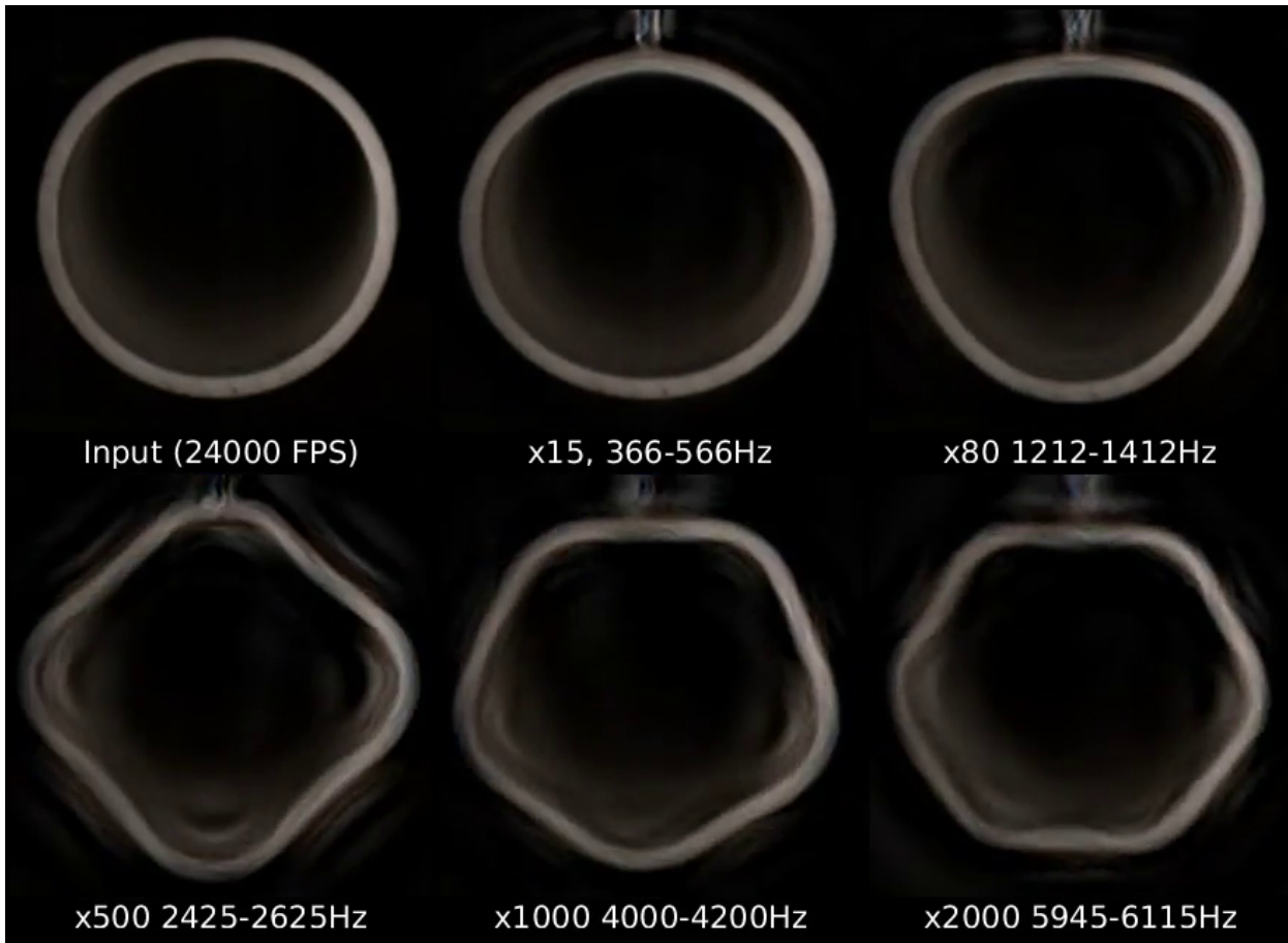
Movie S3. The input pipe video concatenated with five motion magnified videos revealing different modal shapes of the pipe. The sub-videos were scaled up using bicubic interpolation by a factor of 50%. The video was recorded at 24,096 FPS and played back at 30 FPS.
